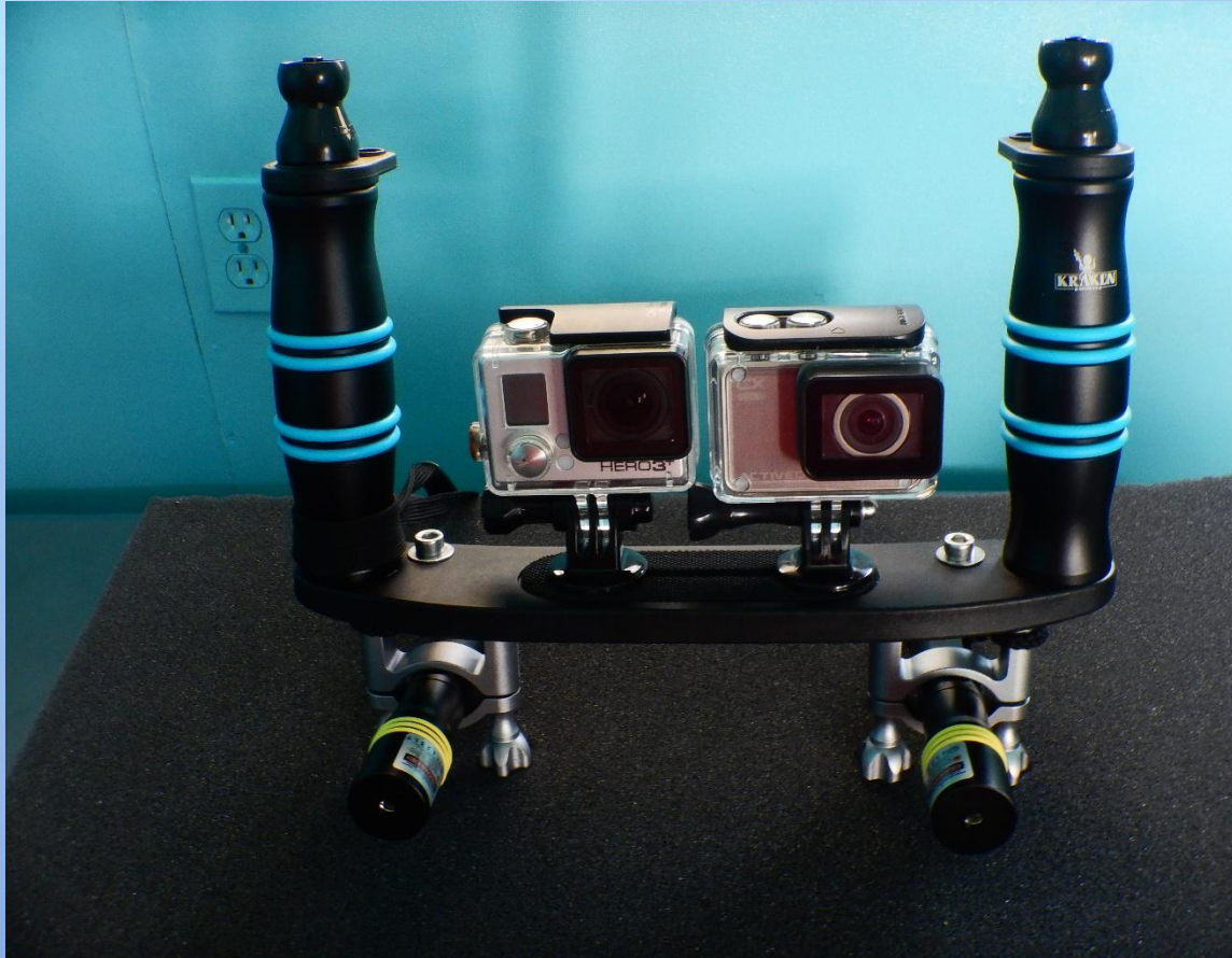
Laser caliper array with two submersible GoPros and twin submersible lasers fitted to a tray with handles. The fixed distance between the lasers (calibrated to 18cm) allows fish length to be estimated with high accuracy from video footage. © A. Tewfik/WCS
